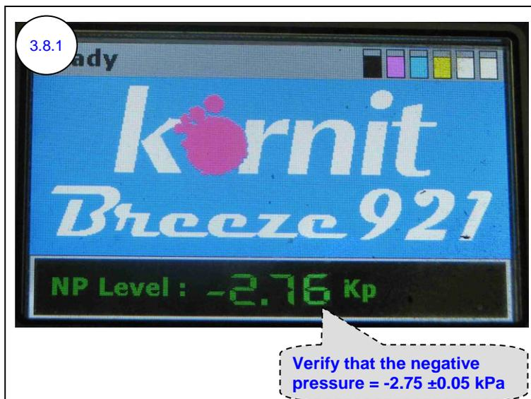
Verify that the value of the negative pressure, as shown on the maintenance panel LCD, is approximately  $-2.75 \pm 0.05$  kPa.
